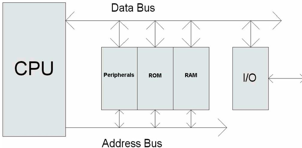
All of the devices that are outside the CPU appear in a single, unified Address Space. In our case, addresses are 16-bits wide, and so the address space is 64K words large.
